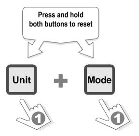
When an error is noted in the operation of the motor unit (indicated by a <u>Flashing RED light</u> on the wall plate or status indicator), the unit can be "Reset" by forcing a re-initialization via the remote control.
