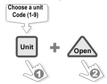
The first time the "Unit" button is pressed the remote displays 1 for the unit code. Each successive press will increase the unit code until it reaches 9.
