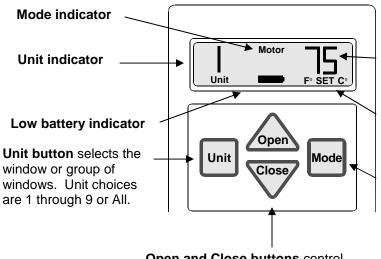
**Open and Close buttons** control windows or blinds. They will also stop the window or blind in a partial open position by pressing the button opposite window or blind travel
