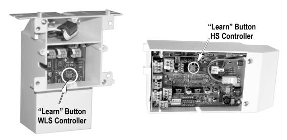
The RF Remote Status LED in the control box will light a steady red and the Motor Status LED (on control board for HS model and wall plate for WLS model) will begin to flash Green. This indicates that the controller is in "Learn" mode.
