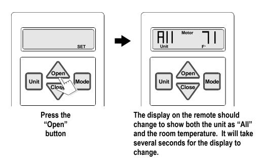
5. Press the "Unit" button on the remote to select the desired Unit Code that will correspond to this window or skylight.
