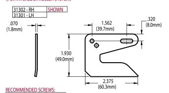
WOOD/PVC/METAL: 2 - #8 PHILLIPS, PAN HEAD, SST SCREWS (LENGTH AND THREAD TYPE TO BE DETERMINED BY PROFILE)
