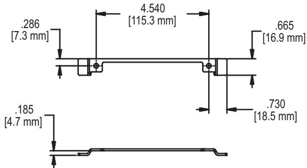
FIG. 6 TRACK & SLIDER ASSEMBLY 11576.XX
